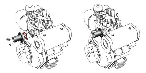
8. Slide a new Gasket P1132 & Intake Adaptor E1146L055 over the 3 Intake Manifold studs and secure using the 3 off retained M6 nuts..
