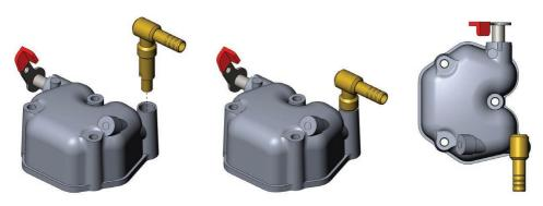
6. Bond Elbow E1223X into the air vent stack. The Elbow also plugs the airway to the cylinder head. (Loctite, 638 retaining Compound, SF764 Activator and SF7063 cleaner recommended). Ensure that the side air vent hole in the Elbow aligns with the cross drilling in the rocker cover. This will leave the hose tail pointing directly forwards, towards the air intake filter.
