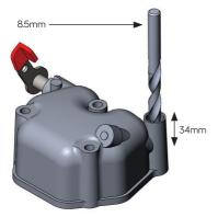
5. Drill down from the top of the air vent stack, 8.5mm dia x 34mm deep. CLEAN OUT SWARF.
