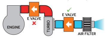
Turbocharged Engines with Intercooler: fit the valve upstream (air filter side) of the turbocharger. If this is not possible the valve may be fitted downstream of the intercooler only if the hose adaptor size for the valve is not too restrictive.
